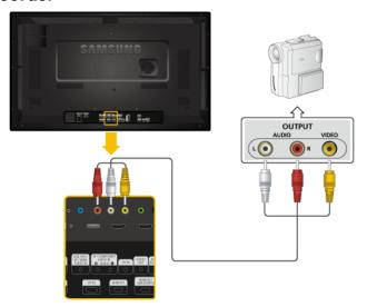
Locate the AV output jacks on the camcorder. They are usually found on the side or back of the camcorder. Connect a video cable between the VIDEO OUTPUT jack on the camcorder and the [AV IN] on the LCD Display.
